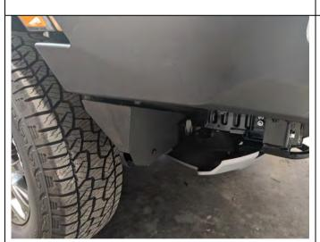
Fasten panel onto wheel intrusion bar using M8 hardware supplied in 3540310 and retighten factory M12 bolt.
