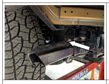
77. Loosen outermost M12 bolt on wheel intrusion bar on both sides.
