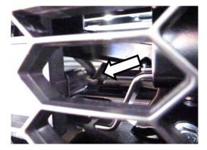
54. As the bar is being offered up to the vehicle, locate and connect the OE radar harness to the connector on the back of the radar unit.
