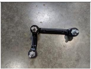
5. Remove captive bolt assembly from each side of the chassis rail.
