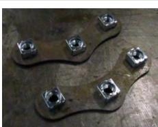
25. Fit 3 x M12 cage nuts to each of the cage nut plates as shown.
