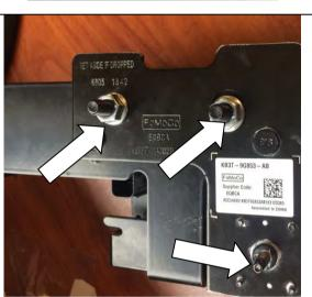
26. Fasten factory radar bracket with radar in place to ARB radar bracket using M8 fasteners sets as shown.
