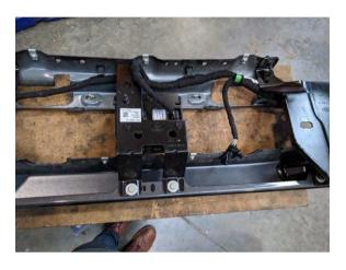
8. Carefully remove 4x front parking sensors and wiring harness from steel bumper and set aside.
